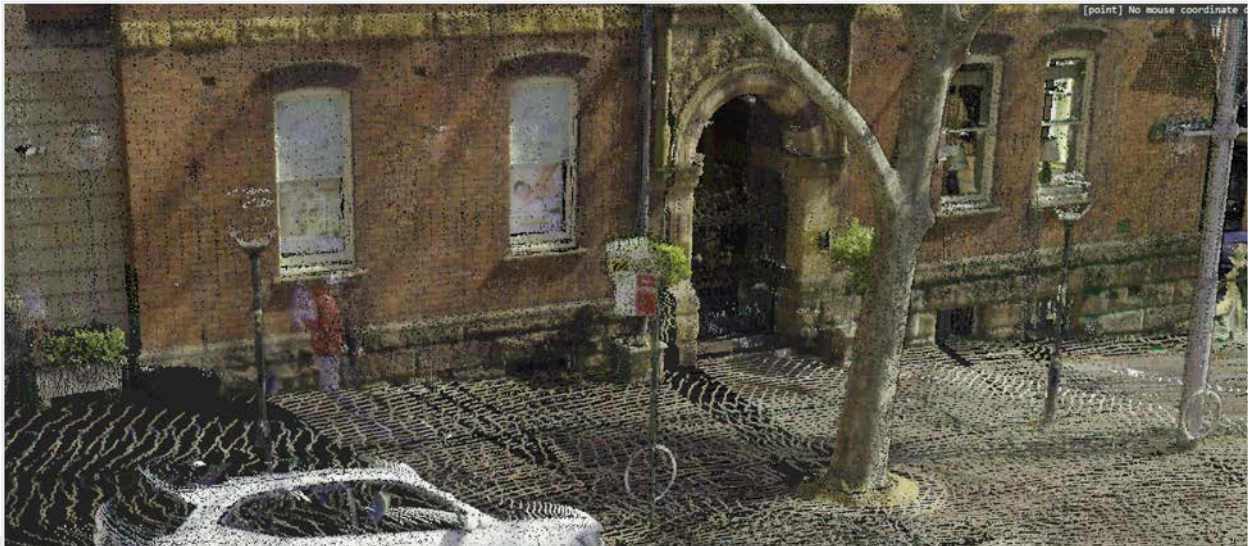
Figure 5b – Detailed LEICA point cloud provided by CMS Surveyors - Path, tree and front entrance of No.93, Macquarie St.
